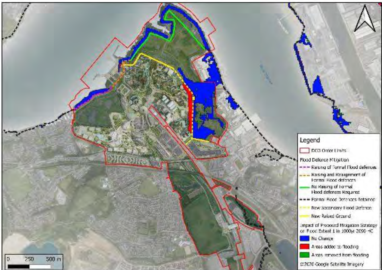
Figure 4-20: Breach 21 in the new secondary flood defence, 1 in 1000 year 2090 higher central climate change projections
