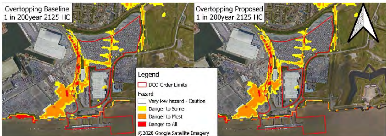
Figure 4-17 Essex Project Site 1 in 200 year Proposed 2020 model compared to Baseline 2020 model during overtopping 2090 using the higher central climate change allowance hazard flood map based on the obstruction greater than 50% manning's roughness value
