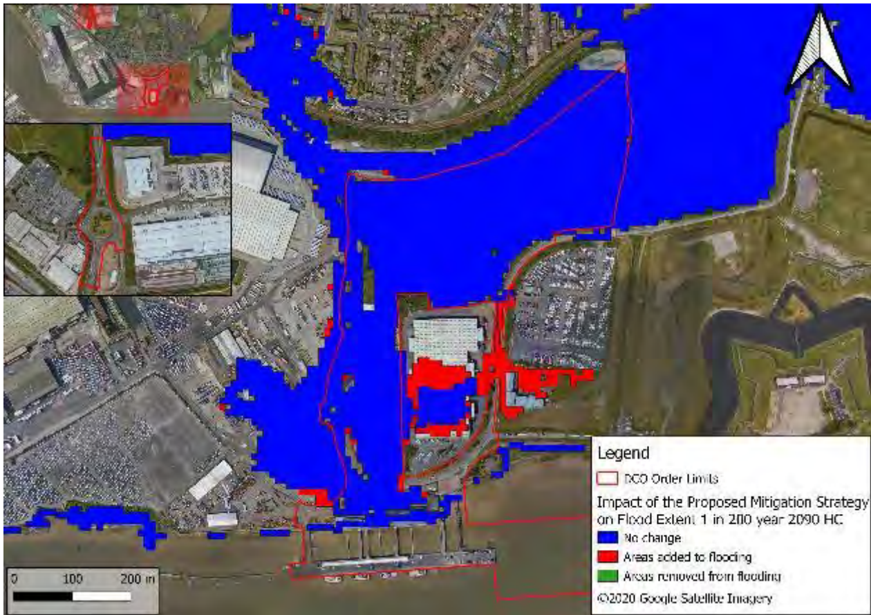
Figure 6-10 Essex Project Site change in Proposed 2020 model compared to Baseline 2020 model for Breach flood extent in the 1 in 200 year event for 2125 higher central climate change projection
