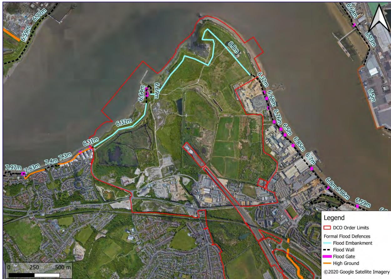
Figure 4-2: Kent Project Site (Main Resort) existing flood defence alignment, type and crest elevation as defined by the data supplied by the EA.
