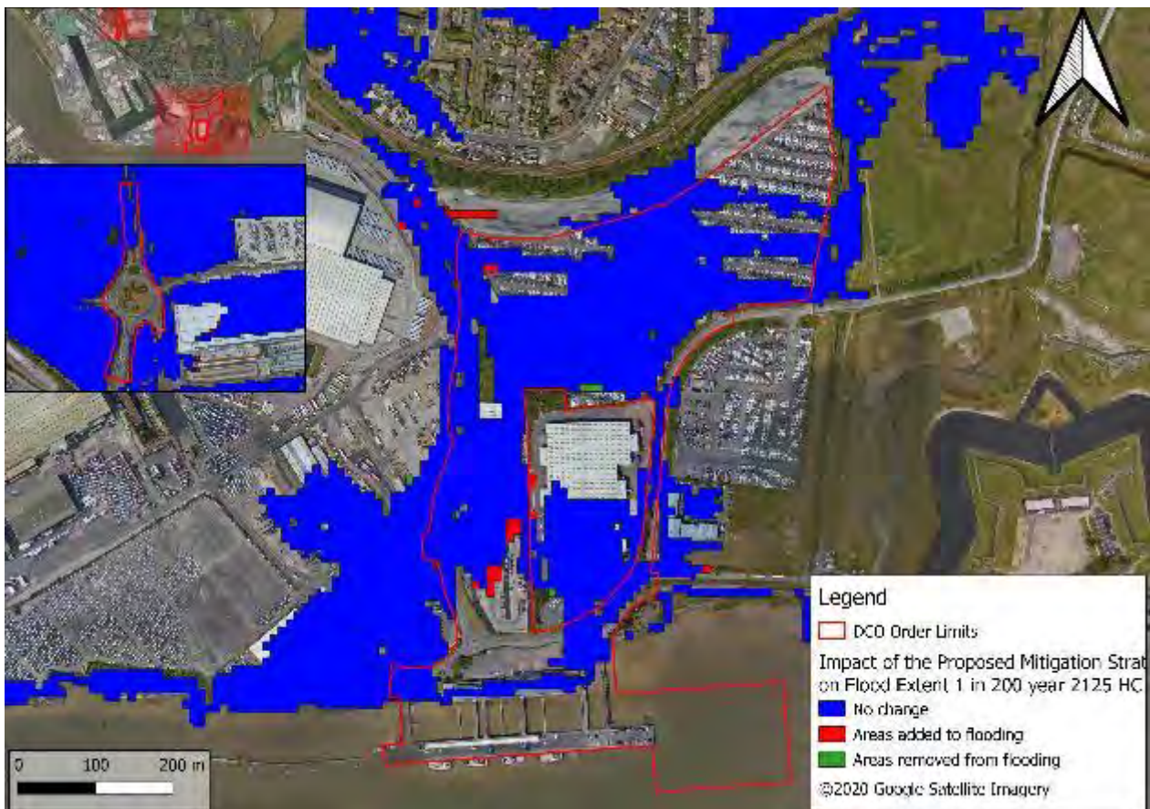
Figure 6-9 Essex Project Site change in Proposed 2020 model compared to Baseline 2020 model for overtopping flood extent in the 1 in 200 year event for 2125 higher central climate change projection
