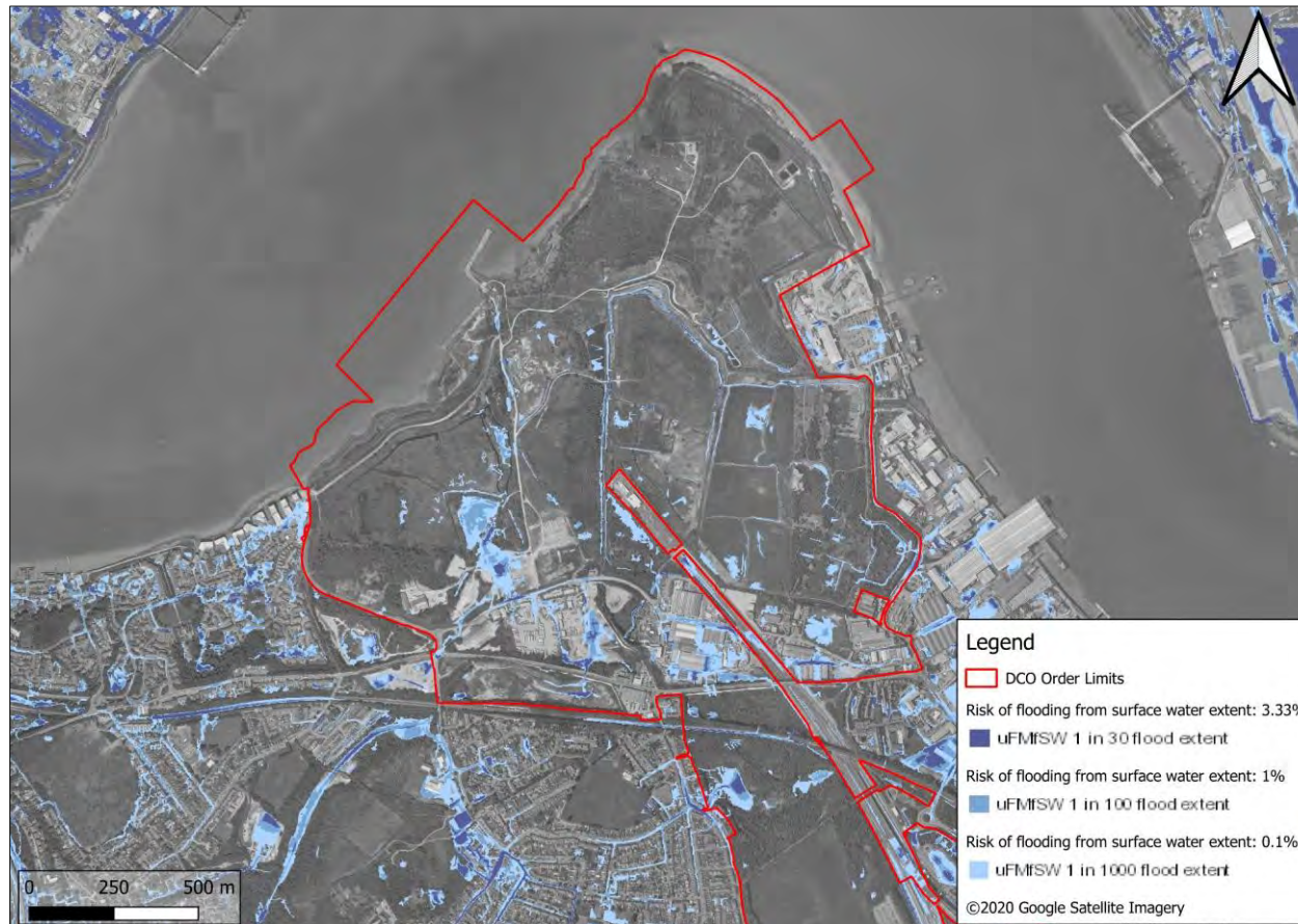
Figure 4-26: EA flood map showing surface water modelled flood extent (Map data ©2015 Google, © Environment Agency copyright and/or database right 2014. All rights reserved. Some features of this map are based on digital spatial data from the Centre for Ecology & Hydrology, © NERC (CEH). Soils Data © Cranfield University (NSRI) and for the Controller of HMSO 2013)
