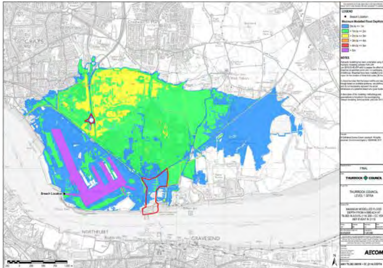
Figure 6-18: Essex Project Site flood risk from artificial sources: Tilbury Docks Breach 3 . DCO Order Limit shown in red.
