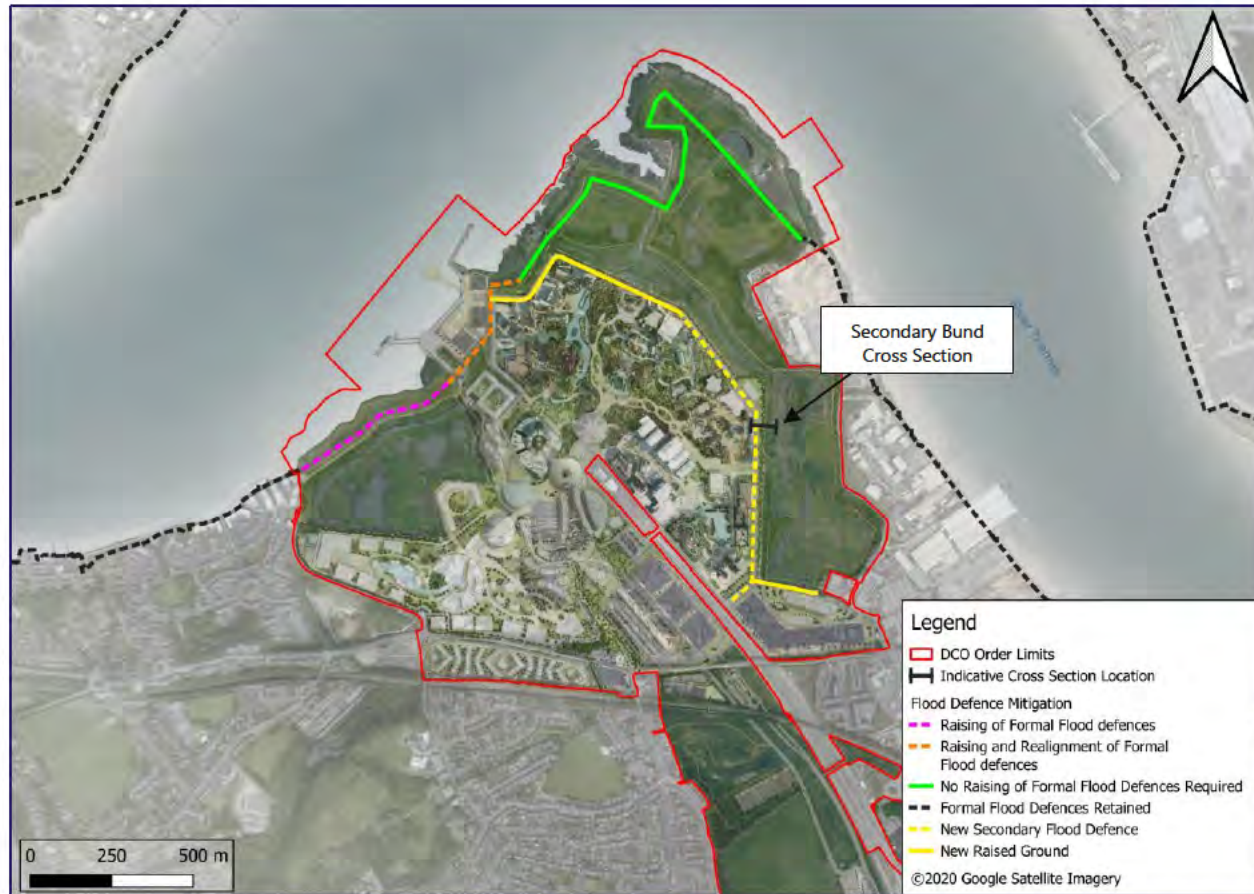
Figure 4-15: Flood Risk Mitigation Kent Project Site (Main Resort) secondary flood defence bund
