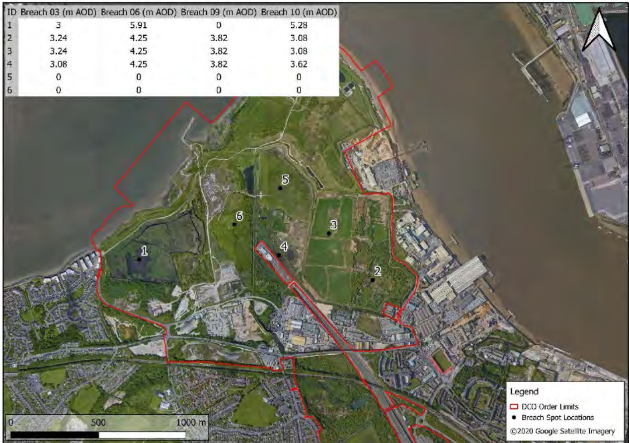
Figure 3-18: Breach analysis water level comparison for the 1 in 1000 year 2090 event, using the higher central climate change projection
