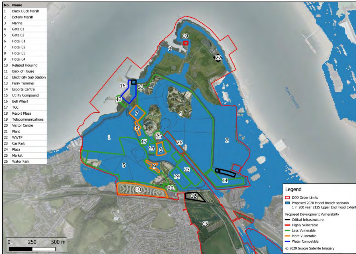
Figure 4-20: Kent Project Site (Main Resort) breach 1 in 200 year event 2125 epoch using the higher central climate change projection flood extent using baseline topography.
