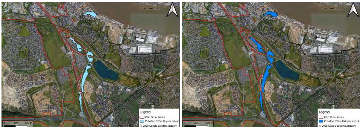
Figure 5-4: Ebbsfleet 2016 model results extents for the 1 in 20 year return period event (left) and the 1 in 100 year return period event (right)
