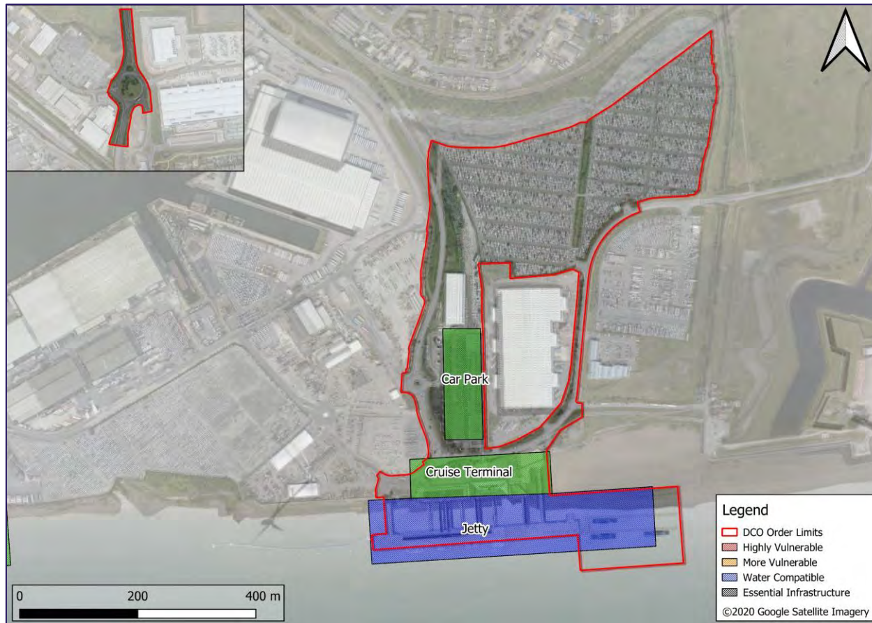
Figure 2-3 Proposed development components of the Essex Project Site and their vulnerability classifications
