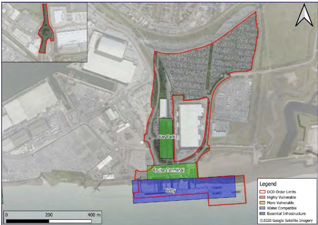
Figure 2-5 Proposed development components of the Essex Project Site and their vulnerability classifications
