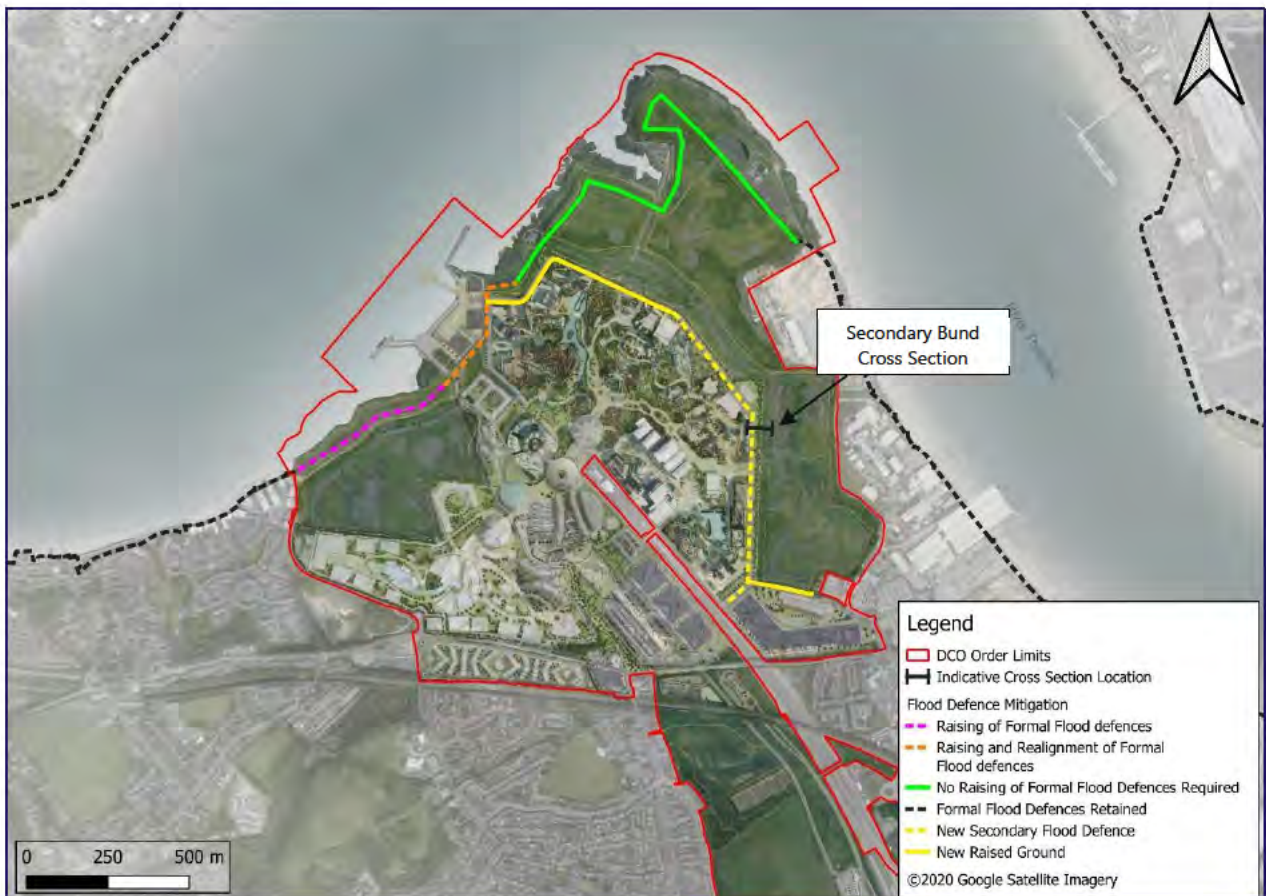
Figure 4-2: Flood Risk Mitigation Kent Project Site (Main Resort) secondary flood defence bund
