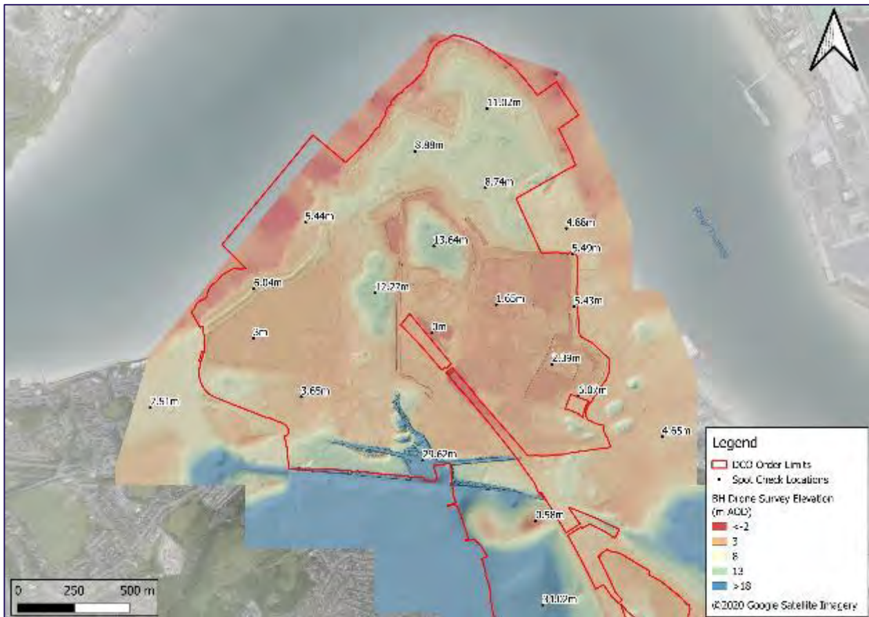
Figure 1-3: Existing flood defence alignment and crest levels for the Kent Project Site (Main Resort) taken from EA data with spot elevations from topographic survey flown July 2020.
