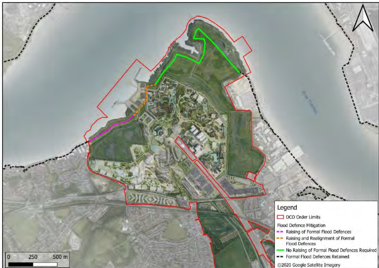
Figure 4-1: Flood Risk Mitigation Kent Project Site (Main Resort) proposed works to the formal flood defences.
