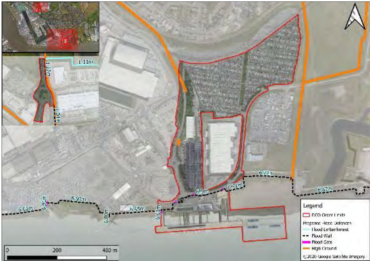
Figure 6-11: EA proposed flood defence alignment information taken from drawing TEA-3F-00.00-DR-CI-00-000005 Rev P04 (January 2018) Illustrative masterplan shown on imagery.
