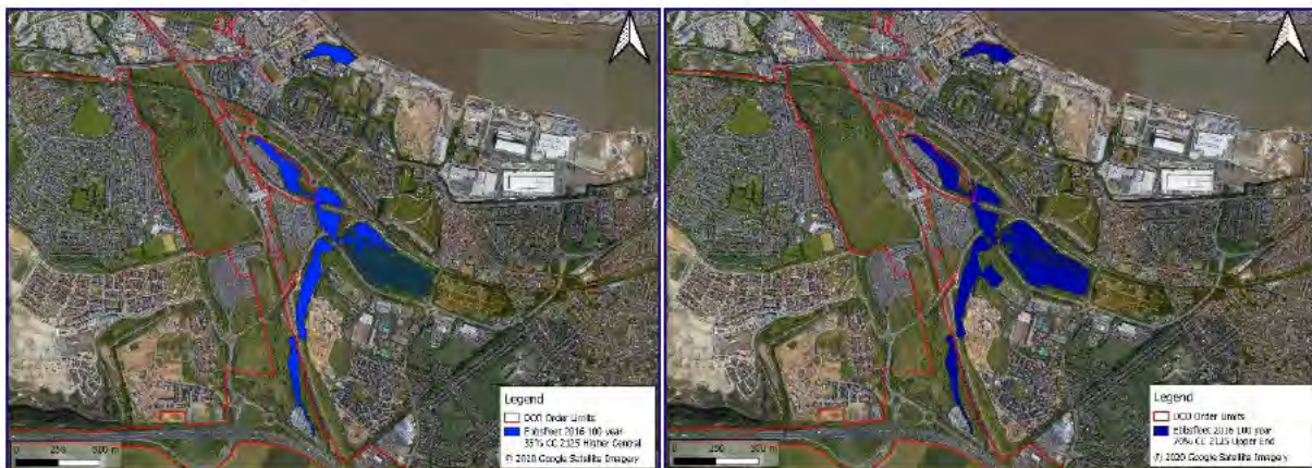
Figure 5-5: Ebbsfleet 2016 model results extents for the 1 in 100 year return period event with 35% climate change 2125 future epoch using higher central sea level rise projections (left) and 1 in 100 year return period event plus 70% climate change 2125 future epoch using Upper End sea level rise projections (right)
