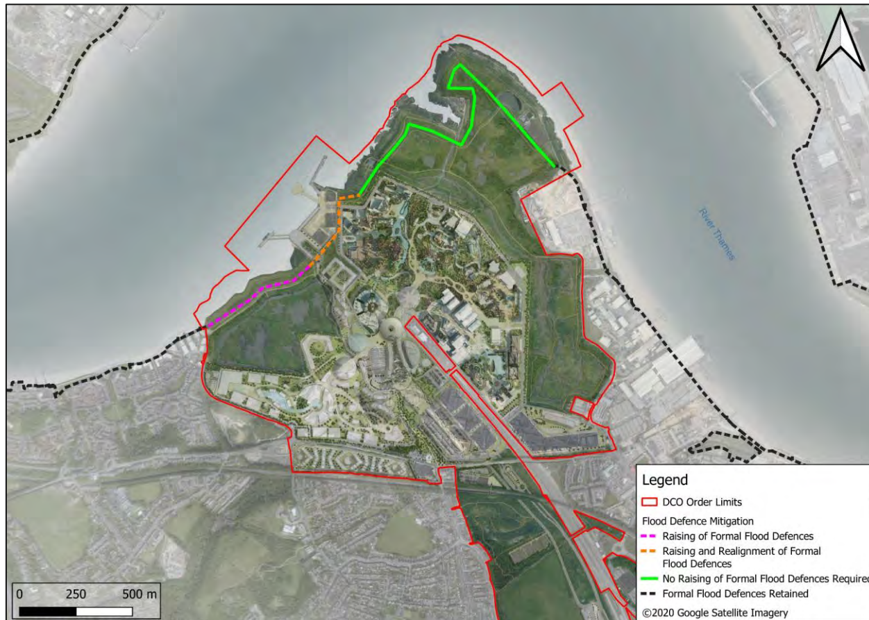
Figure 4-9: Flood Risk Mitigation Kent Project Site (Main Resort) proposed works to the formal flood defences.
