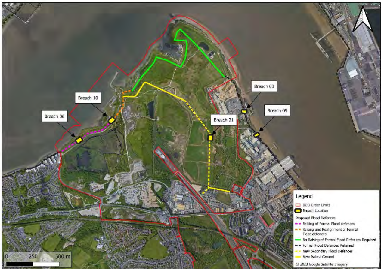
Figure 4-7: Kent Project Site (Main Resort) breach locations
